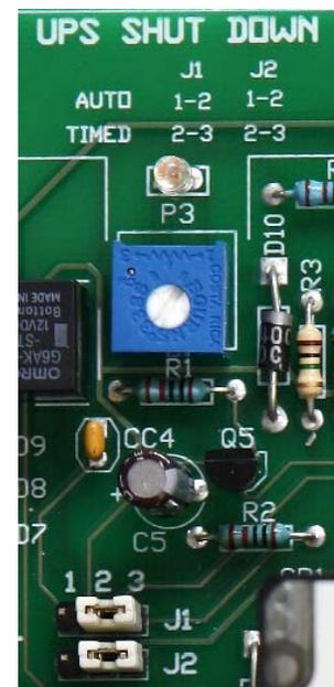
Regardless of the mode selected, this controller has an **LED** above **P3** that will be ON when the failsafe has been shut down after a power failure, and it will remain ON until normal power is restored.
